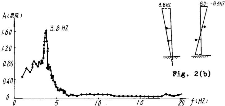
Fig.2(a) Resonance curve of pier caisson
