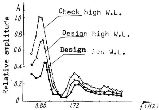
Fig. 4 Resonance curve for various water levels
