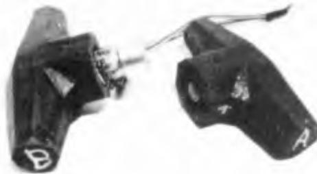
Figure 1. THE LOAD CELL
