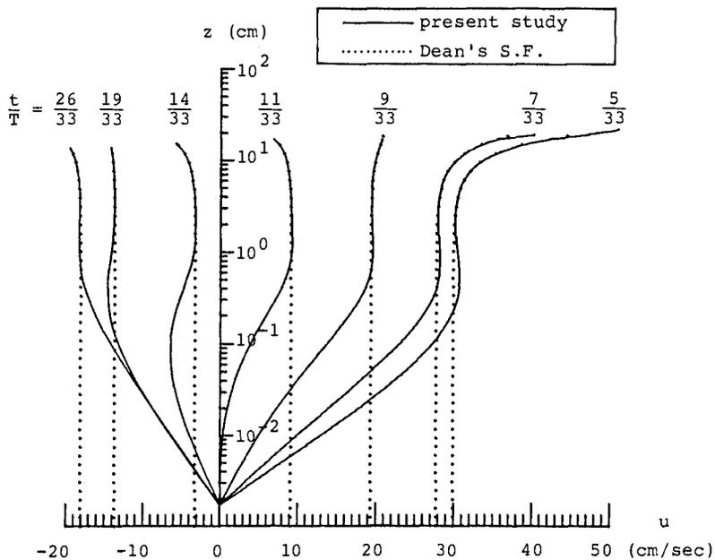
Fig.3 Vertical distribution of velocity profile.
