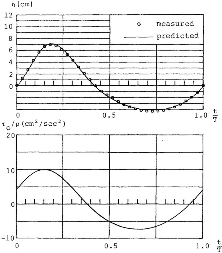
Fig.7 Time-variation of water surface level and bottom shear stress at measured point  $P_1$ .
