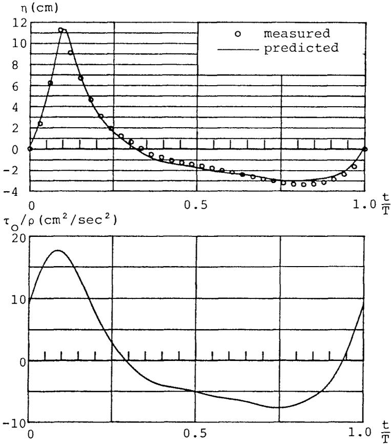
Fig.8 Time-variation of water surface level and bottom shear stress at measured point  $P_2$ .
