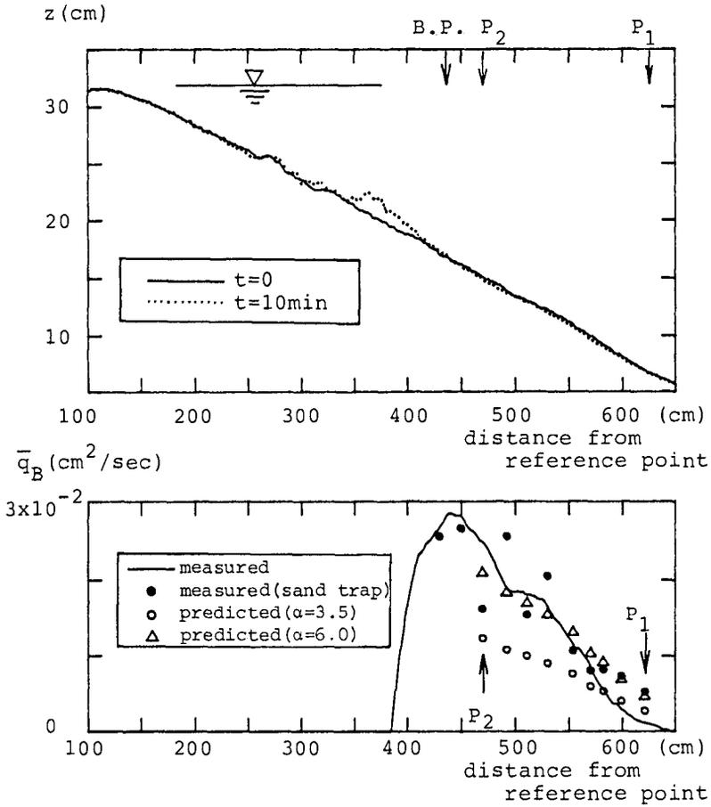
Fig.6 Change of beach profile and bed load transport rate.
