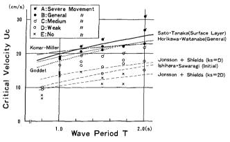
Fig.5 Critical velocity under plane waves
