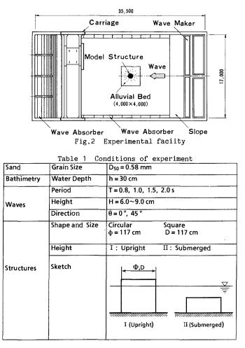
The experiment was carried out in a wave basin  $35m \times 17m$ (see Fig.2) with the water depth kept a 30cm. The model offshore structures, measuring 117cm, were installed on a sand bed  $4m \times 4m \times 1cm$ . The grain size of the sand was chosen as large as D<sub>50</sub>= 0.58 mm with quite a uniform distribution, with the shingle material to be used in the scour protection in mind, and also giving the sand function as a tracer.
