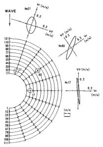
Fig.14 Lissajous figures of bottom velocity vector around a cylinder(Circular -I)
