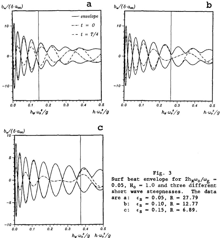
In Fig. 3 the total slope length has been kept constant and the position of the breaker point varied. The reflection coefficients of up to 28 show a significant amplification of the set down wave. On
