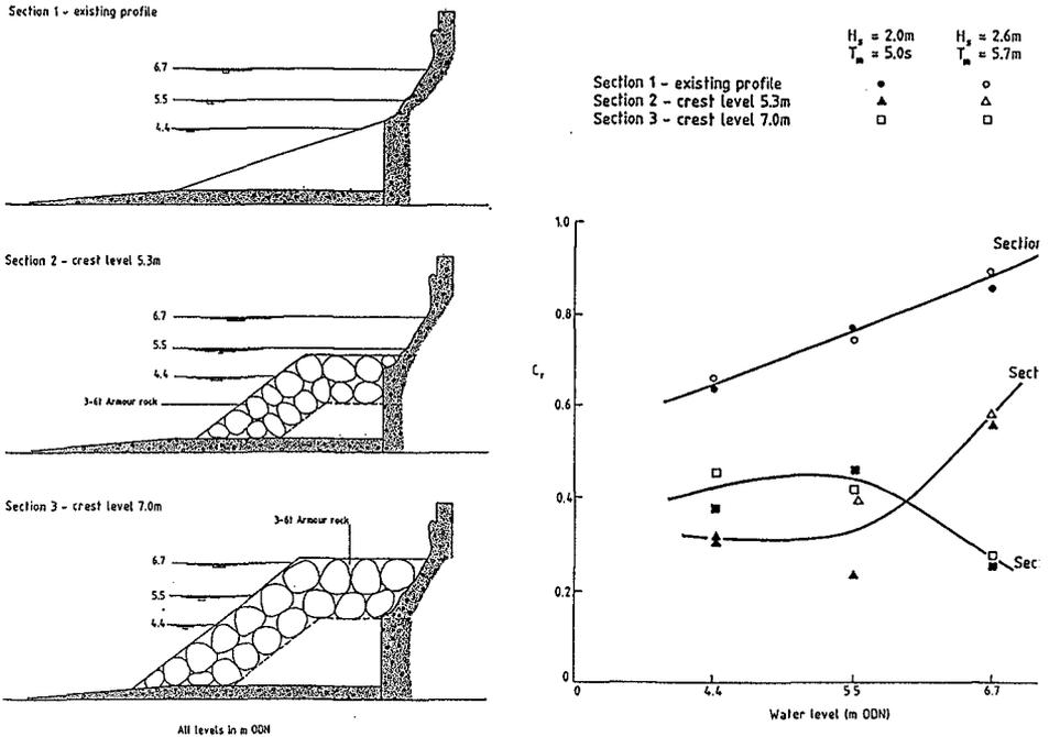
Fig 7 Performance of rock protection to existing wall
