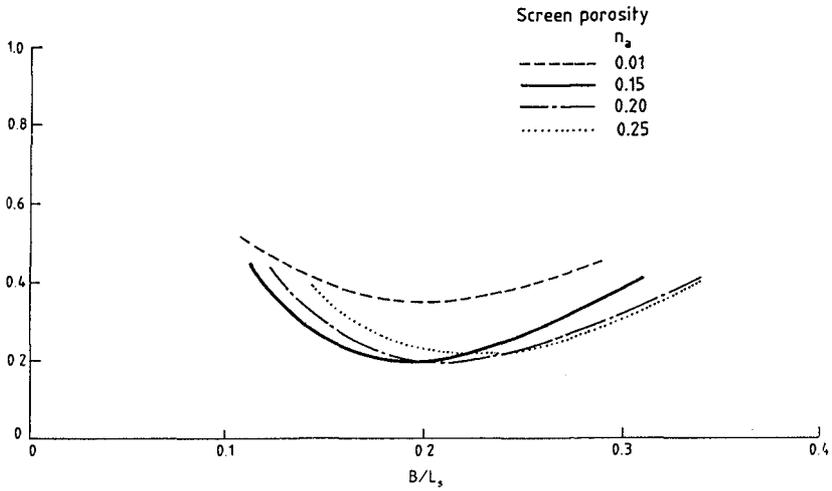
Fig 9 Wave reflection performance of wave screen with impermeable rear wall
