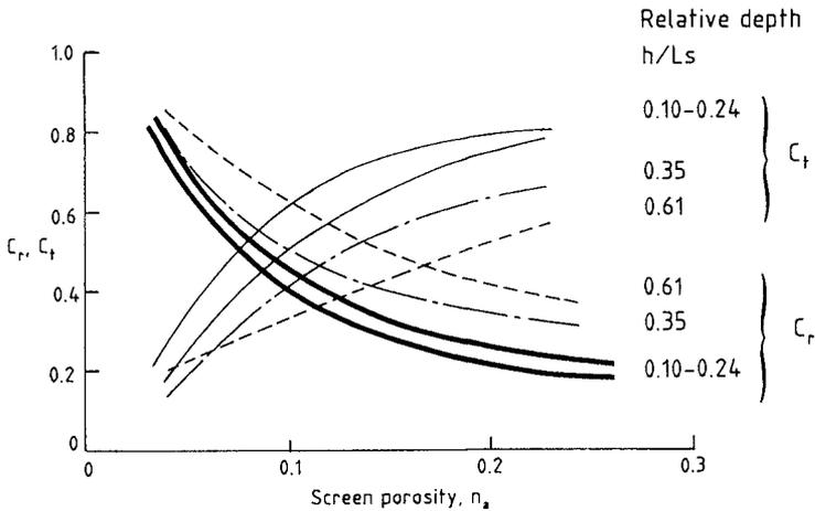
Fig 8 Reflection and transmission for single wave screens
