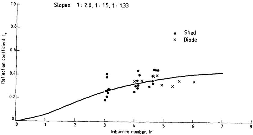
Fig 6 Reflection performance of Shed or Diode armoured slopes, random waves
