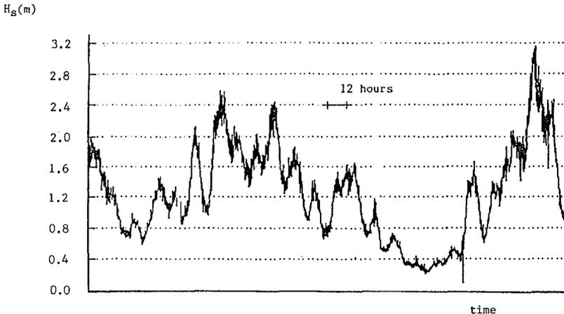
Fig. 1 Measured significant wave heights  $H_s$  at the southern North Sea, platform Euro-0, 50 km west of the entrance to the port of Rotterdam, water depth 26 m. Illustration provided by the Ministry of Public Works and Transportation, The Netherlands.
