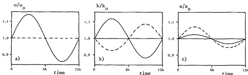
Fig. 2 Results of calculations with simple one-dimensional model for monochromatic waves, tidal period 12 h,  $\omega_0 = 2\pi/10$  rad/s,  $d_0 = 25$  m,  $A_d = 1$  m and  $A_U = 0.63$  m/s. —  $d\omega/dt$  given by equation 6, - - -  $d\omega/dt = 0$  a) normalized absolute frequency  $\omega/\omega_0$  b) normalized wavenumber  $k/k_0$  c) normalized amplitude  $a/a_0$ .
