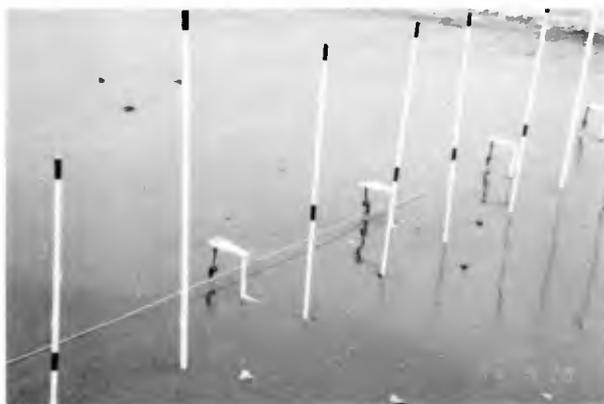
Photo 1 Run-up meter and stick array.
