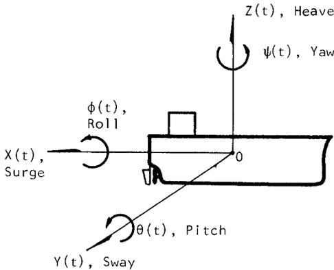
Fig. 2 The definition of six ship motions
