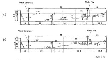
Fig.4 Cross sections of the wave tank
