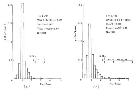
Fig. 13 Frequency of wave forces
