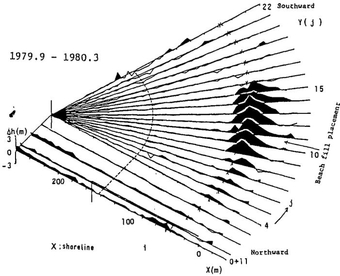
Fig. 8 Change of water depth took place during Sept., 1979 and March, 1980 when borrow sand of 16845m<sup>3</sup> was placed around shoreline between surveying lines No.7 and No.15 at Asakawa-Beach
