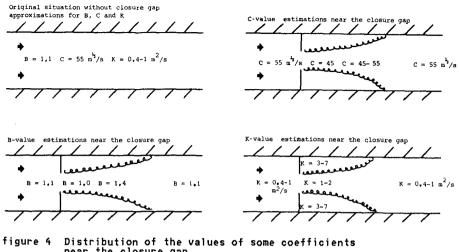
near the closure gap note: Given C-value corresponds to water depths of the channels at compartmentation dam site
