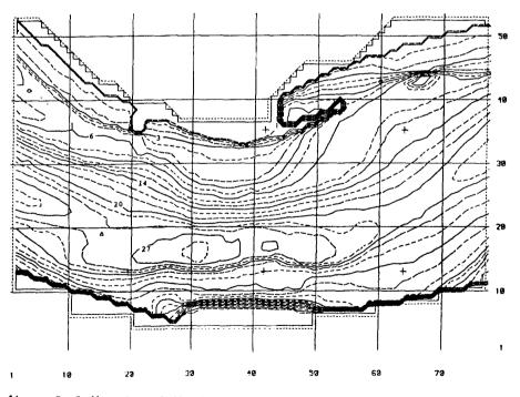
figure 5 Bathymetry of the test model
