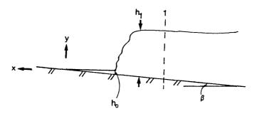
Figure 4. Simplified Model of a Transition from Bore to Run-up Mode.
