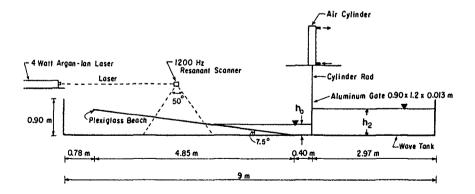
Figure 2. Schematic Drawing of Wave Tank
