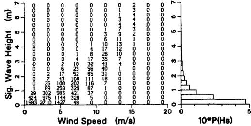
Figure 2 Long-term wind and wave histograms and joint distribution from recorded data and by estimation.
