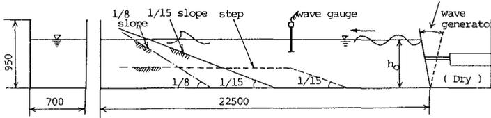
Fig.8 Schematic view of experimental set-up
