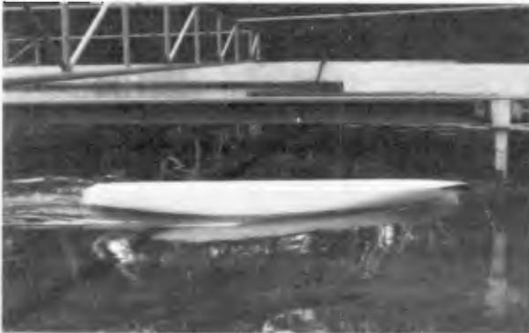
Fig.1 Model Ship Towed by Carriage
