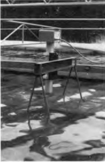
Fig.6 Servo-Type Wave Gage
