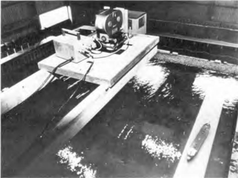
Figure 8. Overhead camera to record model's horizontal excursions
