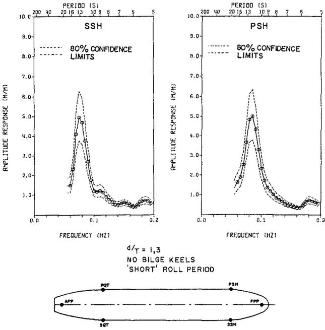
Figure 17. Sample amplitude response functions, 90° wave approach
