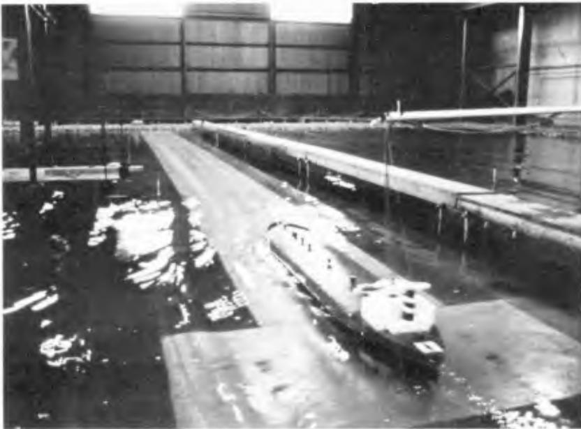
Figure 15. Model test run with  $90^\circ$  wave approach
