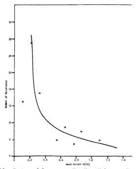
Figure 16. Number of Occurrence Vs. Wave Height at Location #14
