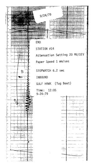
Figure 5. Typical Recorder Trace of Waves from Wake Due to Passage of a Tug Boat
