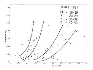
Figure 6. Surge Height Vs. Froude Number at Location #2 for Inbound Ships (Equal Draft)
