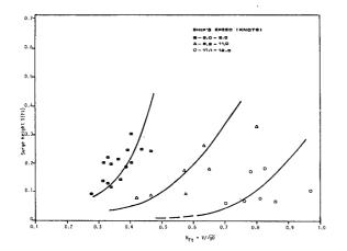
Figure 9. Surge Height Vs. Froude Number at Location #14 for Outbound Ships (Equal Speed)
