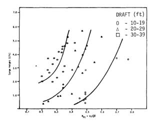
Figure 7. Surge Height Vs. Froude Number at Location #2 for Outbound Ships (Equal Draft)
