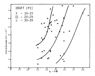
Figure 13. Surge Height/Length of Snip (B.P.) Vs. Froude Number at Location #2 for Outbound Ships
