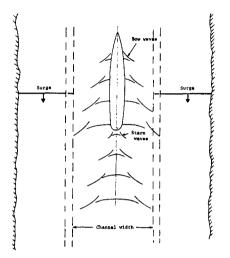
Figure 2. Waves and Surges Generated by a Ship in a Constricted Channel
