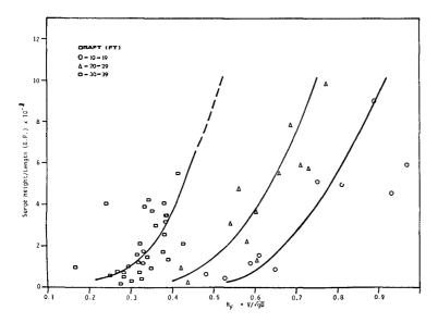
Figure 12. Surge Height/Length of Snip (B.P.) Vs. Froude Number at Location #2 for Inbound Snips
