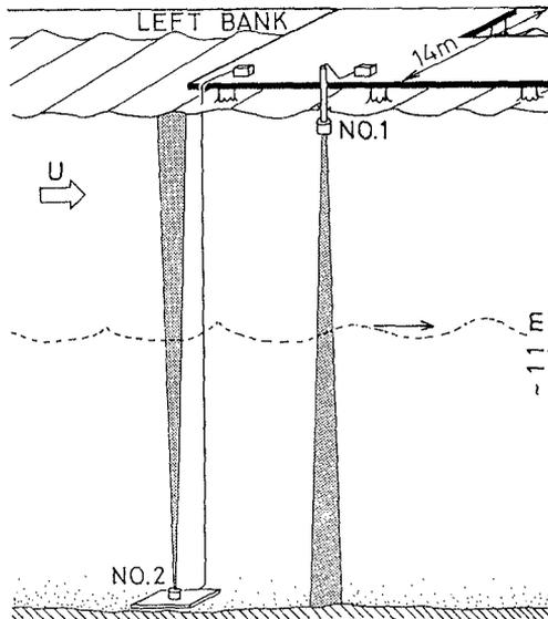
Fig.3 Pier station and two echo-sounder transducers
