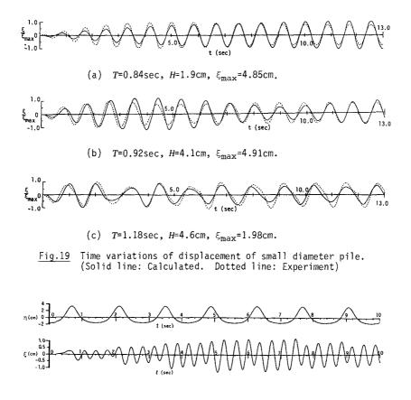
Fig.20 Time variations of hyperbolic waves and the displacement of small diameter pile.
