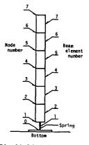
Fig.18 Division of pile into elements.
