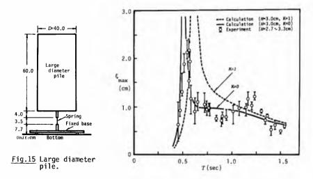
Fig.16 Caracteristics of resonance.
