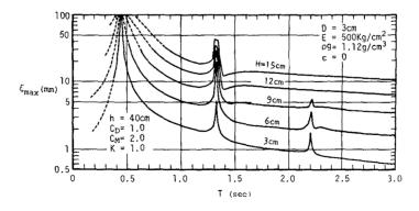
Fig.6 Characteristics of resonance due to small amplitude waves<sup>49</sup>
