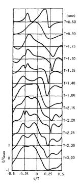
Fig.7 Time variations of the displacement at the top point of cylinder\*).
