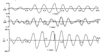
$\frac{Fig.21}{(n: water level variation, \xi: displacement, F: wave force)}$
