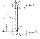
Fig.17 Notation of forces and displacements at beam element.
