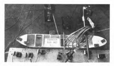
Fig. 7. Instrumentation set-up used in moored seakeeping model study.
