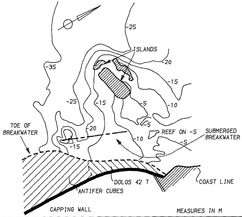
ALIGNMENT SUBMERGED BREAKWATER IN FRONT OF DOLOSSE SECTION
