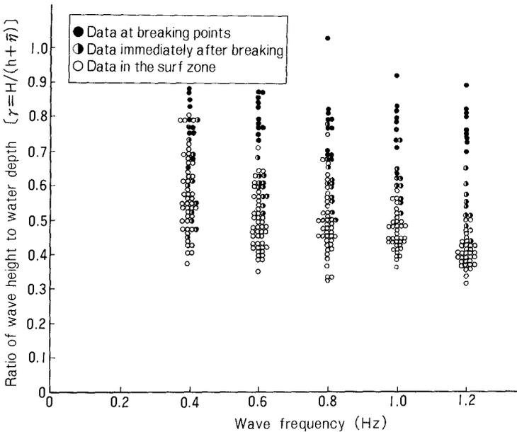
Fig.5 Ratio of wave height to water depth in the surf zone
