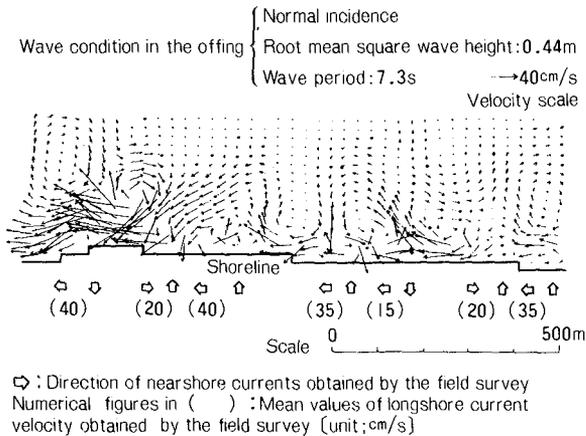
Fig.12 Calculated result of nearshore current pattern
