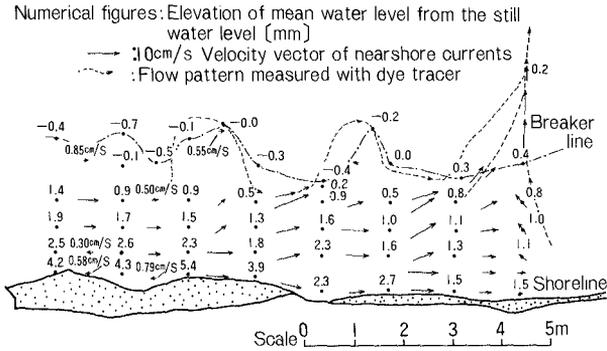
Fig.1 Relation between velocity vector field due to nearshore currents and horizontal distribution of mean water level (Experimental result)
