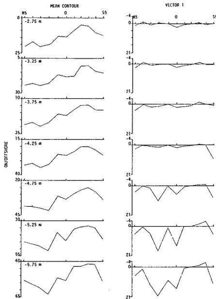
Figure 4. The mean contours and first eigenvectors for each of the seven Siletz Spit contour data sets.
