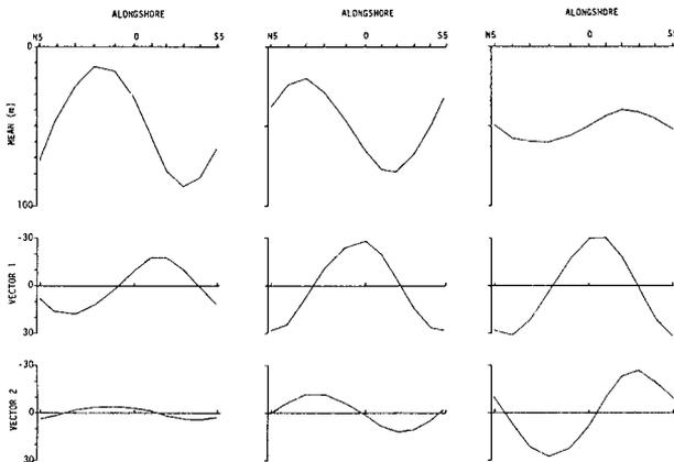
Figure 3. Mean contours and first and second eigenvectors for data depicting a longshore rhythmic pattern with amplitude variations, and a) 90° envelope phase shifting; b) 180° envelope phase shifting, c) 360° envelope phase shifting.
