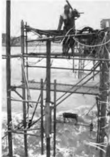
Photo 2 Close-up of surf zone measurement station
