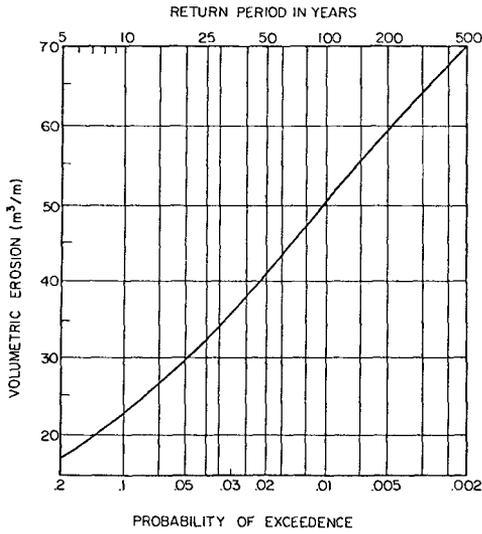
Figure 8. Predicted Frequency Curve for Volume Eroded.
