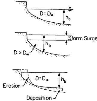
III. SEDIMENT TRANSPORT EQUATION  $Q = K(D - D_*)$
