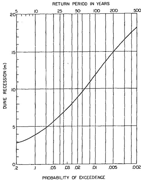
Figure 9. Predicted Frequency Curve for Dune Recession.
