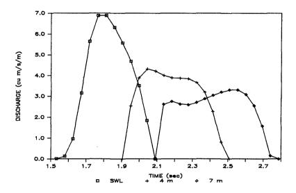
FIGURE 2. Specific discharge at the toe of the dune versus time for three positions of the dune relative to the intersection of the still water level and the beach face.
