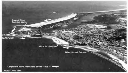
The Tweed River training walls have trapped on Letitia Spit 6.4 million cubic metres of sand that would otherwise have moved northward to the Gold Coast beaches. The construction of groynes at Kirra in an attempt to overcome the resulting beach erosion problem has further interrupted the flow of sand, and has moved the problem area further north.
