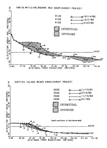
Figure 2. Sediment sampling locations on two of the projects thru time showing the change in intertidal and offshore samples with change in profile shape.
