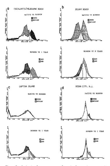
Figure 5. Grain size frequency curves from the four projects comparing 1) the borrow with the native showing the 3 phi cut off and the actual excess fine grain material and 2) the borrow with the one year (8 year for Delray Beach) showing the calculated 3 phi cut off with the actual loss of fine material.
