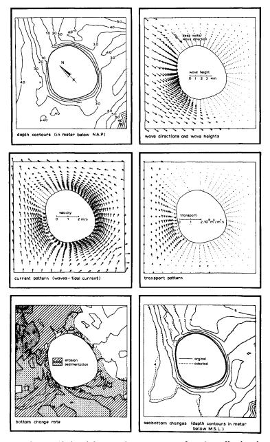
. Fig. 8 Detailed models; results at moment of maximum flood and waves from the North
