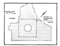
Fig. 5 Small tidal model; results max. flood flow situation
