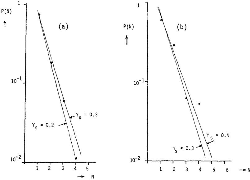
Figure 3 - Group length distribution for  $H_{*} = H_{1/3}$ ; records pooled according to values of spectral estimate of  $\gamma$ . Dots: observed values. Lines: theoretical values of  $\gamma_s$  at the limits of the class interval of the observations. (The lines have been drawn only for the purpose of visualisation; only the values for integer  $N$  have meaning.)
