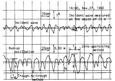
Fig.3 Incident wave and swash oscillation
