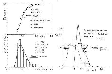
Fig.18 Comparison between measurements and calculations ( Zero-upcrossing method )
