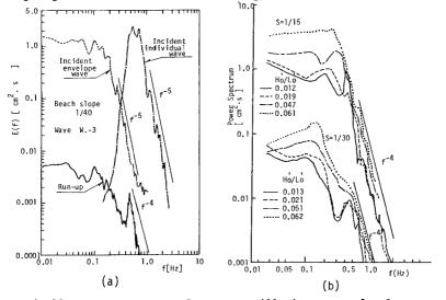
Fig.12 Power spectra of run-up oscillation on gentle slopes
