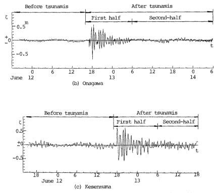
Fig. 2 Time sequence records of water level deduced from tide and tsunami gauge records.
