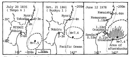
Fig. 1 Tsunami heights and tsunami source areas of the 1835 Tenpo and the 1861 Bunkyu earthquakes inferred from old documents by Hatori (<sup>3</sup>), and the tsunami source area caused by the Off-Miyagi Earthquake in 1978 as defined by Iwasaki and Mano(4).
