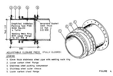
To achieve a seal at the south end of the bridge, the notched end of the pipe was cut off square and a specially designed sleeve was inserted and bolted between the steel pipe flanges. Once the pipe was commissioned, the plastic liner would expand and seal itself against a neoprene ring around the sleeve.
