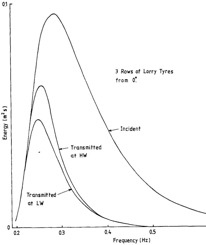
Fig. 4 - Breakwater Performance for 3 rows of lorry tyres with waves from 0°
