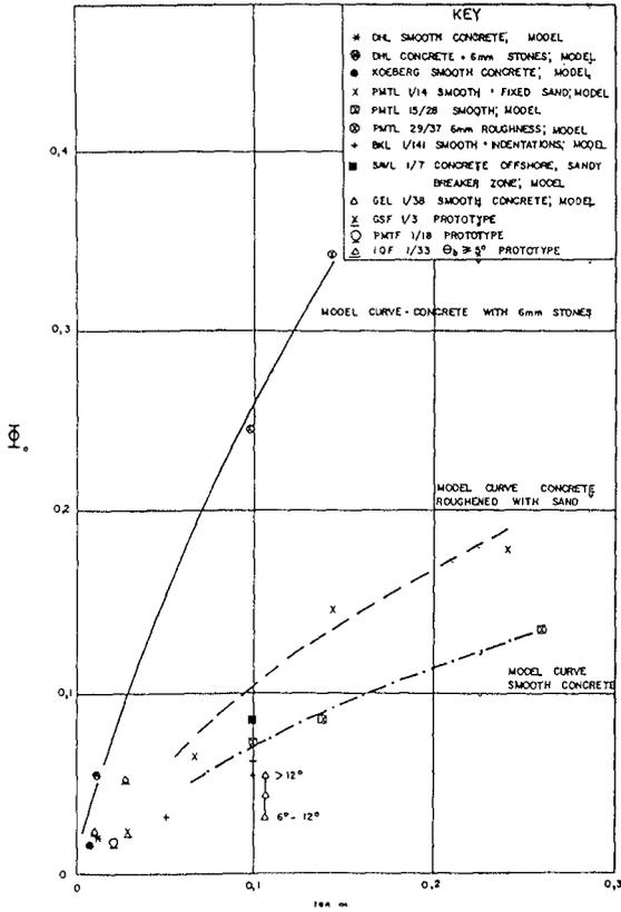
FIG. 1 RELATIONSHIP BETWEEN  $\Phi_b$ , BEACH SLOPE AND BED ROUGHNESS
