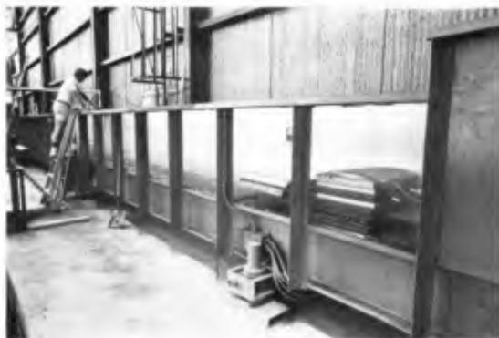
Fig. 2. A View of the Open, Flow Recirculating Flume.
