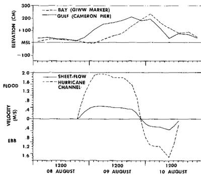
Figure 9. Current velocity simulations for flow across South Padre Island, based on Manning equation. Data from Figure 8A. Flow Regime 1 is for 30-cm deep sheet overwash; Flow Regime 2 refers to 2-m deep hurricane channel.
