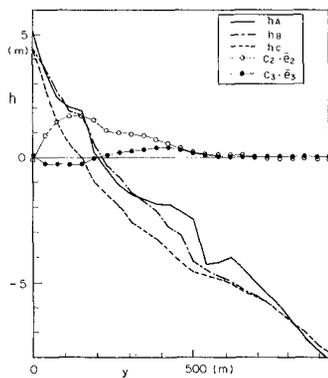
Fig. 14 Comparison of the measured beach profile and that calculated by the products of the eigenfunction  $e_k$  and the function  $C_k$  ( $h_A$ = measured beach profile,  $h_B$ = calculated beach profile,  $h_C$ = mean beach profile,  $C_2e_2$ ,  $C_3e_3$  = variation of beach profile corresponding to the second and third eigenfunctions)
