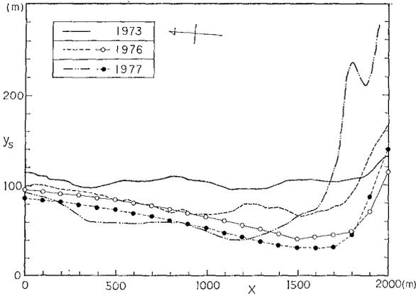
Fig. 7 Results of the shoreline simulation (The calculated shorelines of 1976 and 1977 are indicated by  $\circ$  and  $\bullet$ , respectively. The measured profiles are shown by the solid, broken and chain lines.)
