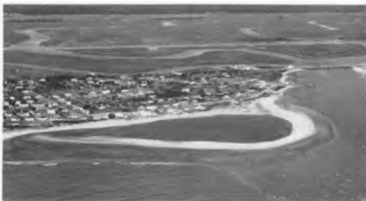
Figure 9. Oblique aerial photograph of the downdrift shoreline of Breaches Inlet, South Carolina. The large bar that has partially attached to the Isle of Palms formed after the ebb-tidal delta had been breached.
