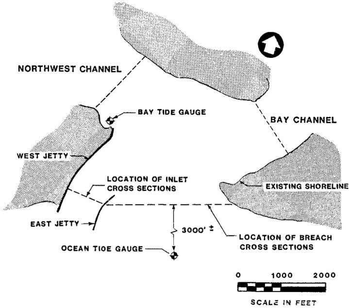
Figure 11 - Inlet Cross-Section and Tide Gauge Locations
