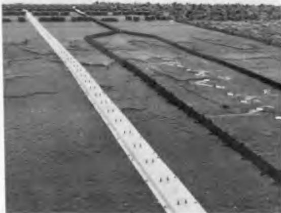
Fig. 1: Wave run-up probe
