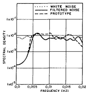
Figure 11 Simulated input spectrum for Table Bay Harbour
