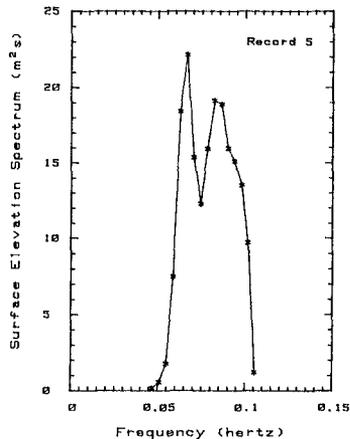
Fig. 6 Typical surface elevation spectrum - Record 5
