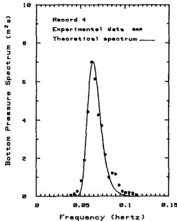
Fig. 8 Comparison of measured bottom pressure spectrum with modified Wallops type spectrum
