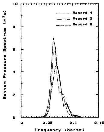
Fig. 4 Bottom pressure spectra showing evolution with time
