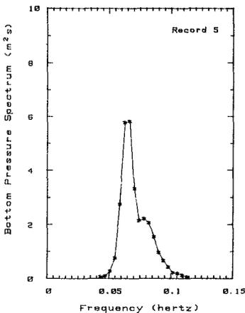
Fig. 5 Typical bottom pressure spectrum - Record 5
