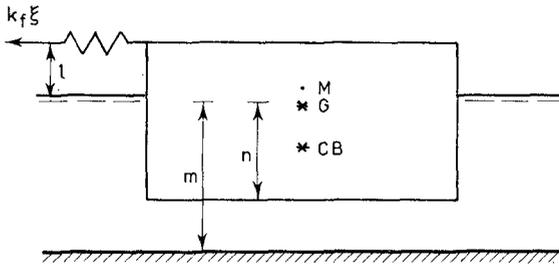
Fig. 16 The geometry of moorings and ship's stability.
