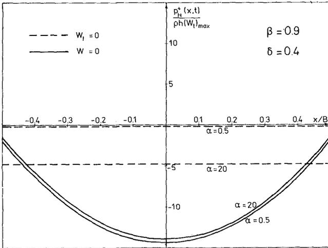
Fig. 9 Pressure variation under the ship induced by a heave motion.
