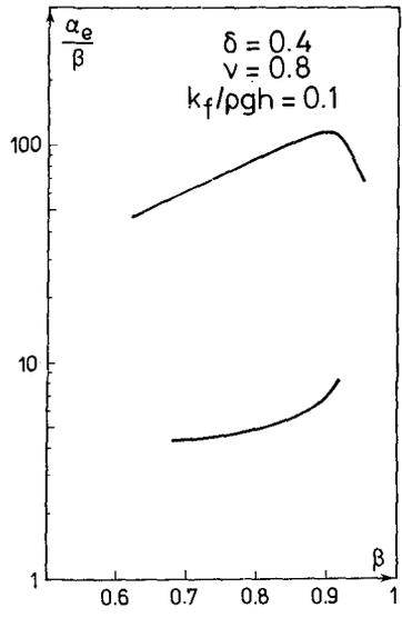
Fig. 17 Resonance frequencies for coupled roll and sway.
