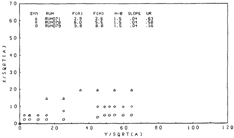
Fig.15 Normalized Jet Trajectory (effect of  $F_0$ )
