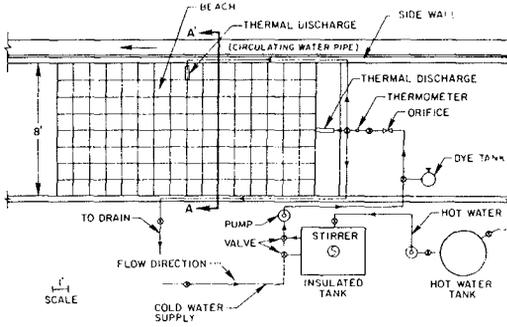
Fig.1 Schematic of the experimental set-up (Plan View)
