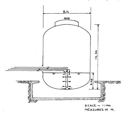
Figure 2. University of Hawaii's Large Circular Testing Tank
