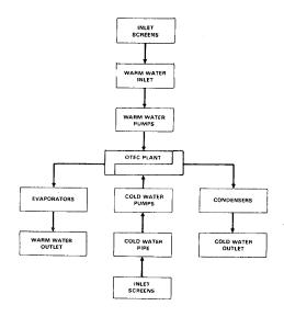
Figure 1. Schematics of OTEC Seawater System (from Richards and Vadus, 1980)
