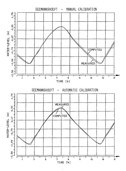
Fig. 5: Comparison Manual to Automatic Calibration
