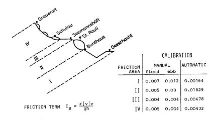
Fig. 6: Friction Parameters after Calibration
