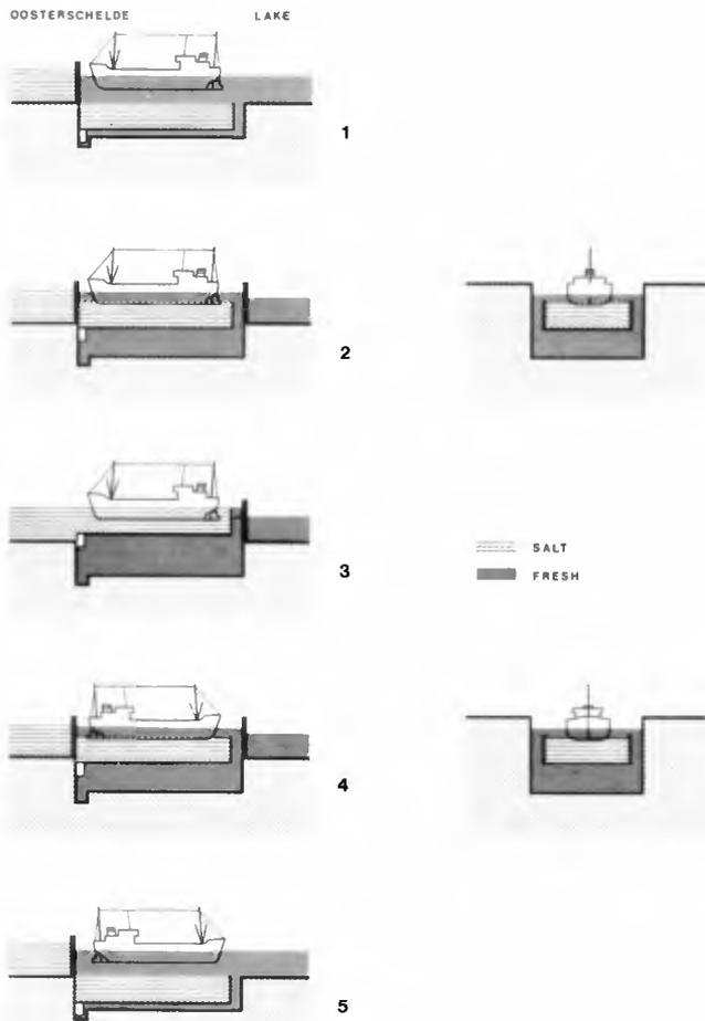
Figure 8: Oosterdam ship lock with vertical shiplift 1-3: Ship traveling from the fresh lake to the salt Oosterschelde, 4-5 ship traveling from Oosterschelde to the lake.
