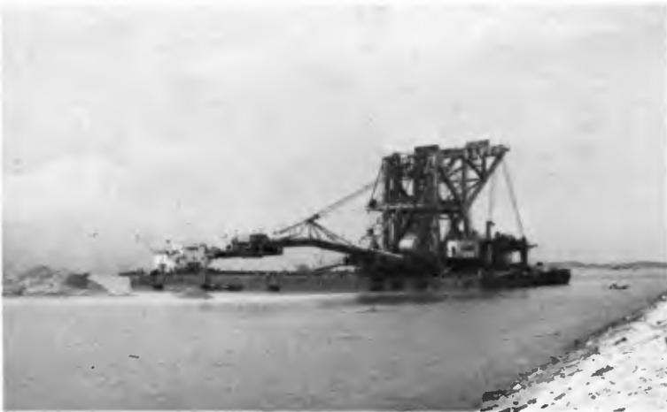
Plate 6. Reclaimer unloading fill material from barge into the sea to form reclaimed land.
